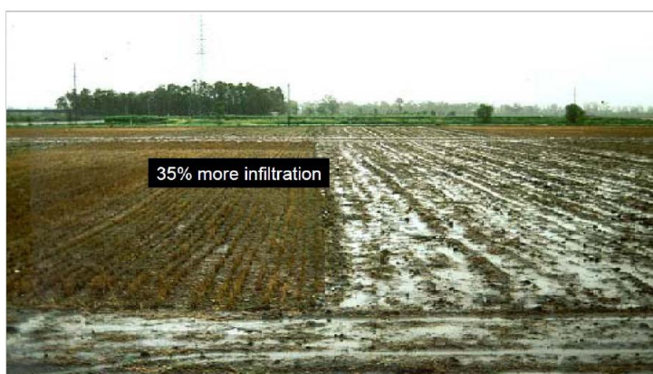
Figure 24b: A dramatic demonstration of the impact of soil compaction. The soil of an experimental plot (Italy) has been subjected to heavier loads on the right-hand side of the image than on the left-hand side. The compacted structure of the soil on the right has resulted in a reduced infiltration capacity of the soil, leading to surface ponding and waterlogging. © Ezio Rusco
